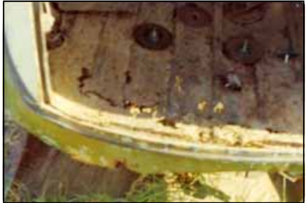
Beaver tail section and boot floor
