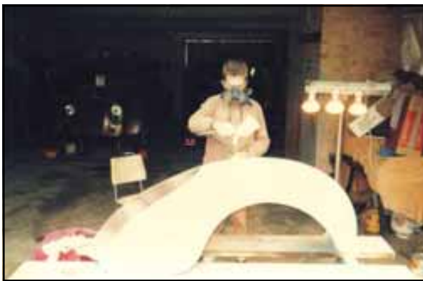
Undercoating front guard
