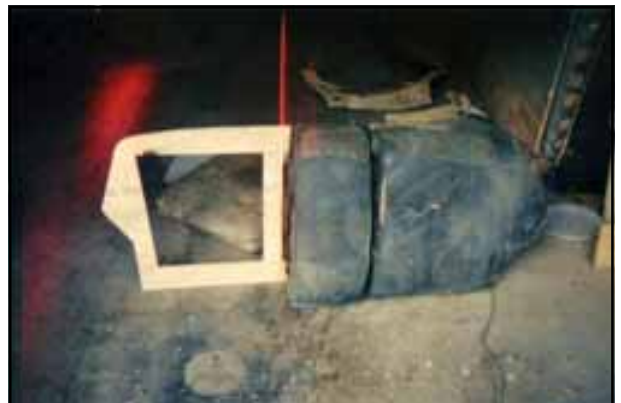
All that is left of the rear seat, complete new frame had to be made.
