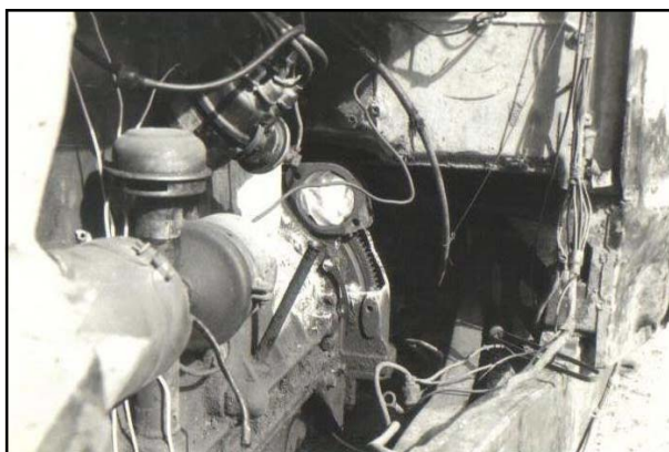
Note chunk out of bell housing
