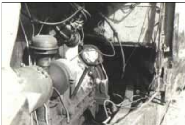
Note chunk out of bell housing
