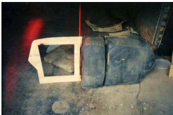
All that is left of the rear seat, complete new frame had to be made.
