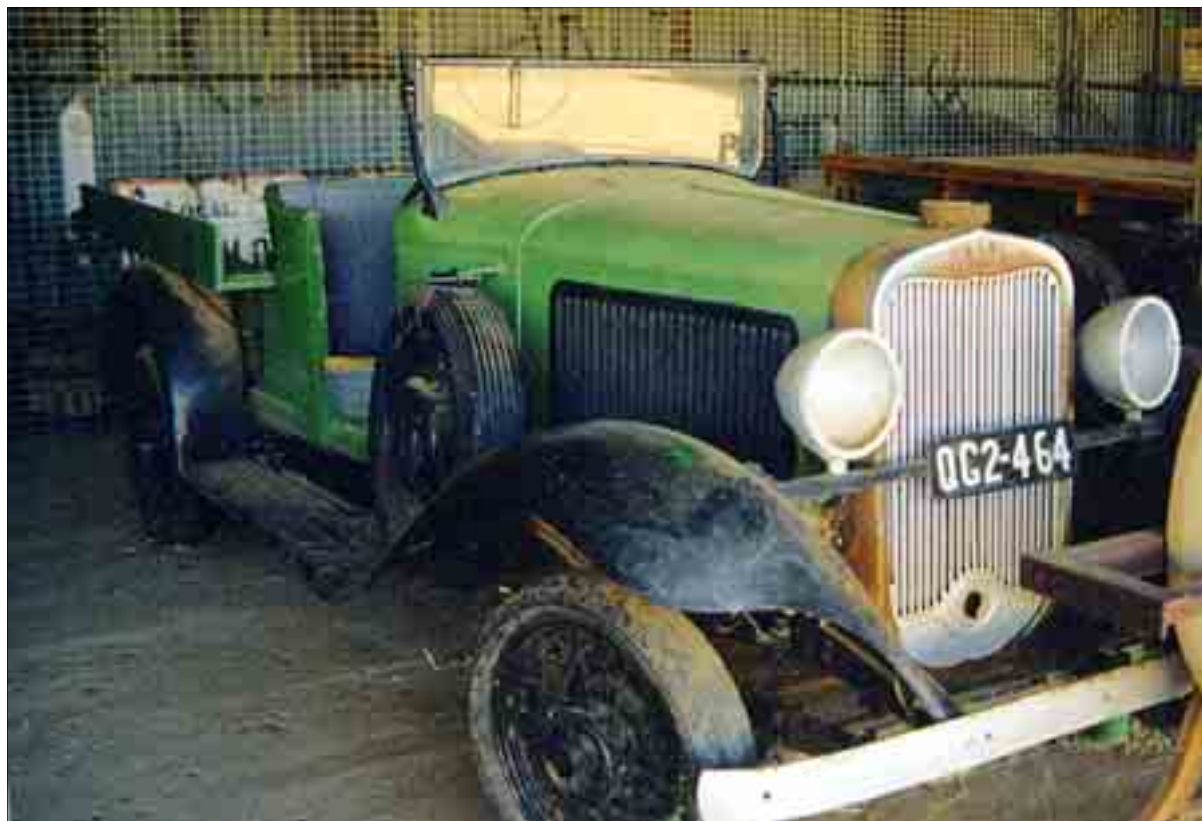
1932 Dodge 4 model DM. Side-valve engine, only 2,000 built, in Windsor Ontario, Canada. Photographed in a museum in Tambo, Queensland.
