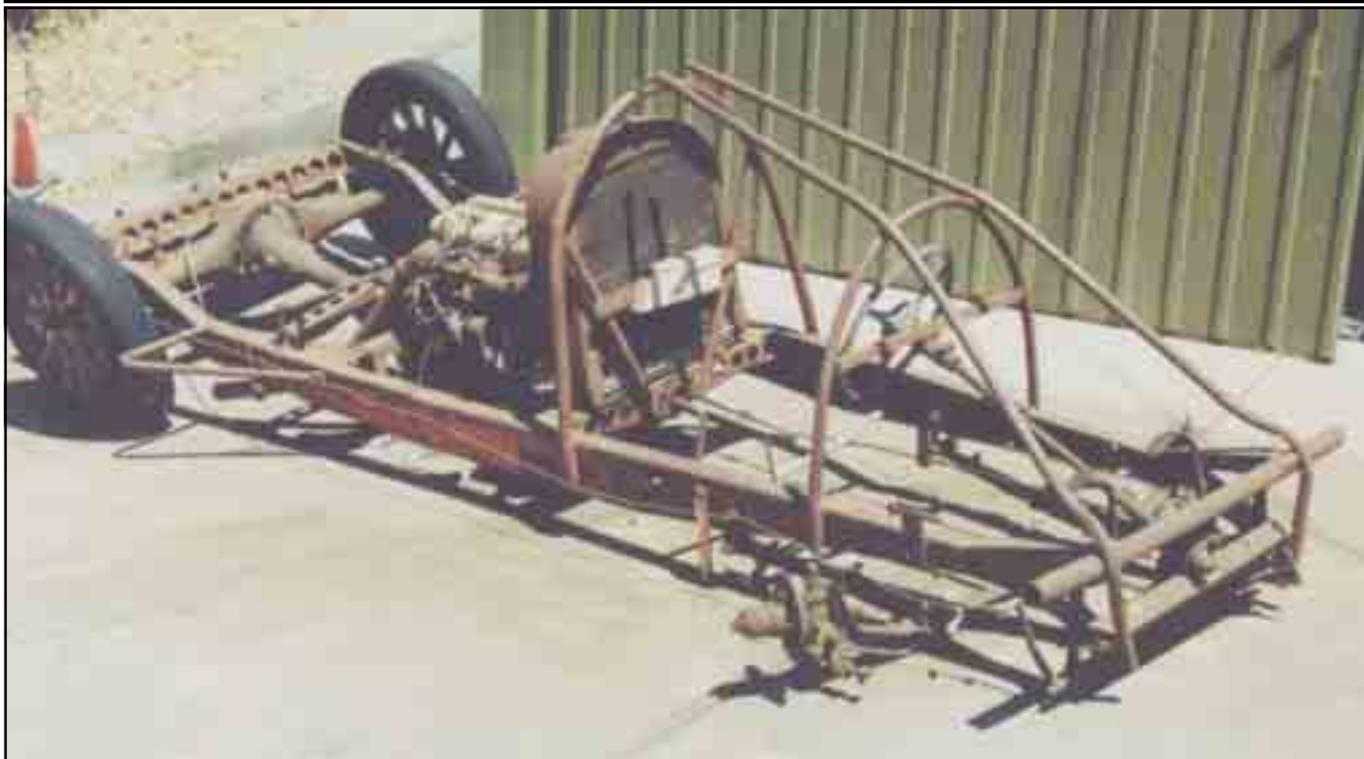
Radiator, motor and gearbox moved back.
