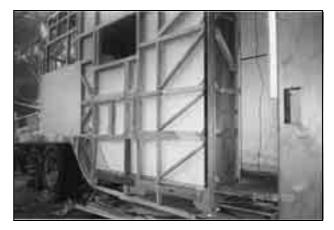
This was the view of the near side prior to cladding. Note how the interior of the kitchen had to be finished before the cladding went on.
