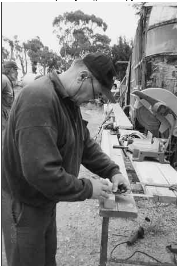
Keith Lucas measures carefully before fitting one of the oregon battens
