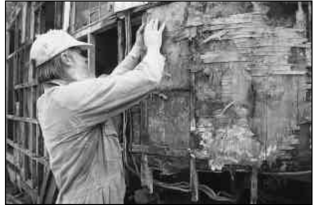
Graham Bailey(above) caresses the newly exposed bitumenous insulation near the front off-side of the caravan but shows a bit more aggression later (below)
